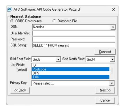
After specifying your database settings, you should click the Connect button where the Wizard will attempt to connect to your database. When successful it will update the fields displayed below. For Nearest to work correctly you need to ensure the correct grid easting and northing fields are selected. These should be on the OS GB grid system. If you need to add grid reference fields to your database and populate it, then please do this prior
